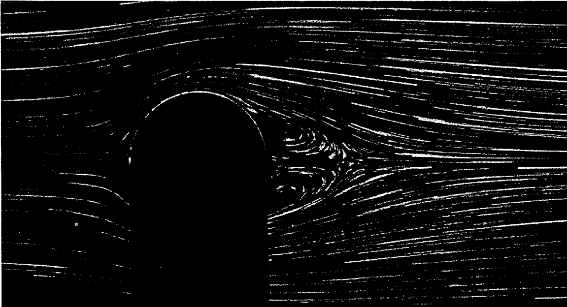
Figure 9. The flow visualization picture of streamlines for Re = 56.5 ( Archives de l'Academie des Sciences de Paris. Payard & Coutanceau 1974 )
