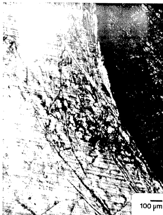
Figure 7. Photomicrograph of Propagating Radial Crack Emerging From Microcracks.
