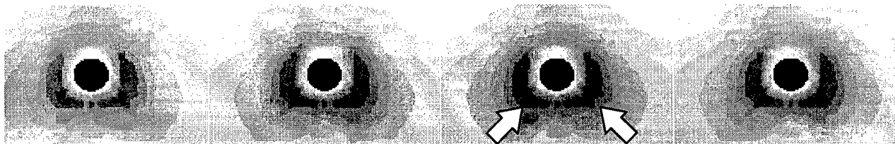
(b) Maximum Principal Stress Location Obtained From Finite Element Analysis.
