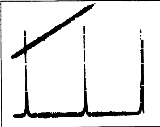
Figure 3. Confocal interferometer trace displaying single frequency output. Upper line displays ramp voltage to interferometer.
