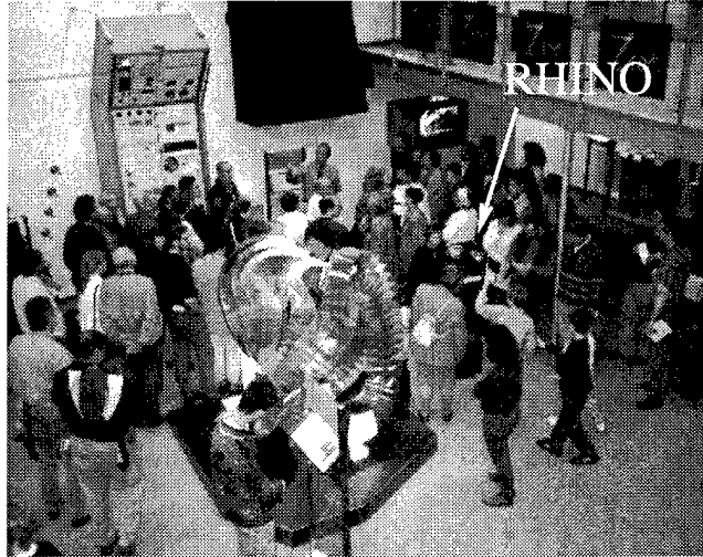
Figure 15: The robotic tour-guide in action, in the “Deutsches Museum Bonn.” To navigating safely through dense crowds while avoiding collisions with “invisible” obstacles (such as a metal plate shown in the center of this image) required accurate maps. The area in (a) measures only 60 by 60 meters, and the total map is only approximately 45 meter long.
