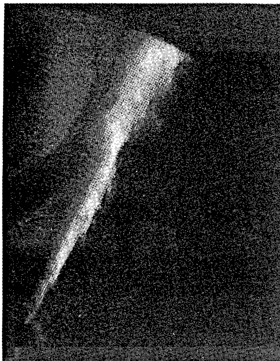
c) Exciplex LIF image of the vapor phase at 1.6 msec after fuel injection
