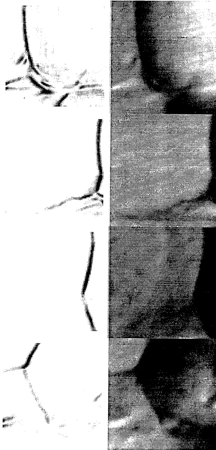
Grayscale contour plots of the density gradients (left hand side) and the density ratio \rho/\rho_0 (right hand side) at 6.8, 10.2, 17.4, and 30.4 \mu\text{sec} for the shots shown in Figure 5. The dark gray indicates high relative densities, while the light gray indicates low relative densities. The density gradient plots are to be compared to the shadowgraphs near the triple point in Figure 5.
