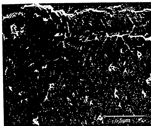
Figure 2. Scanning electron microscope image of InN grown by crystallization from a nitrogen saturated indium melt.
