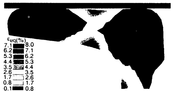
Fig. 2 - V-SEP seal after crushing: constant equivalent deformations on deformed geometry.
