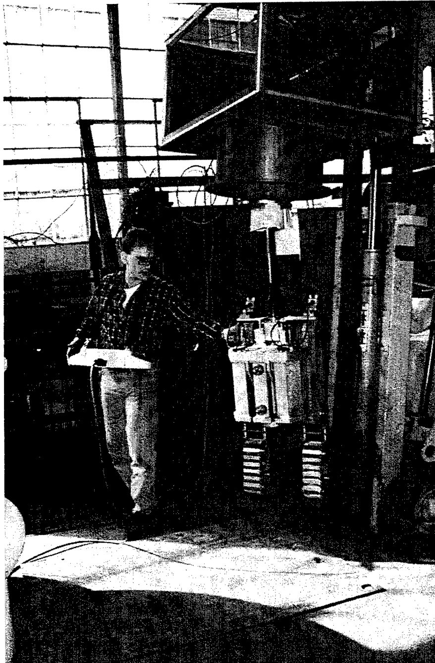
Figure 13. Crawler hanging by tether during acceptance test at CMU.
