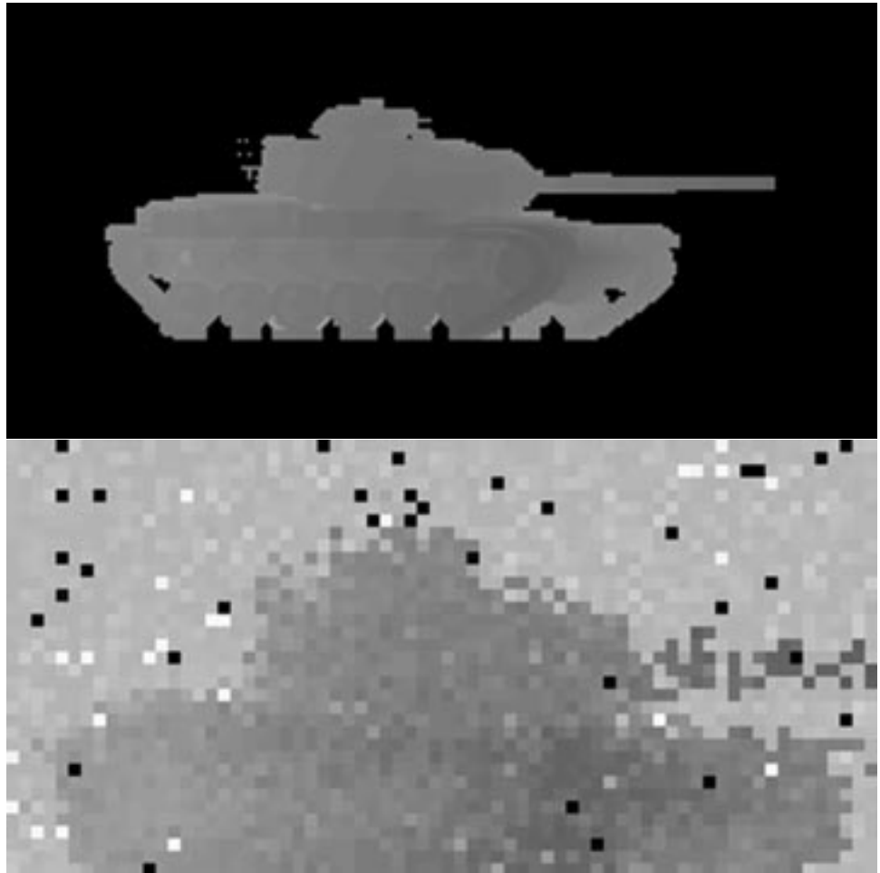
Figure 4. Input range image and resulting ladar image. (Black pixels indicate dropouts and white pixels indicate anomalies.)
