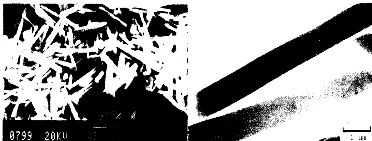
Fig.7 Morphology of needle-like mullite quenched from 1150 to 0°C.
