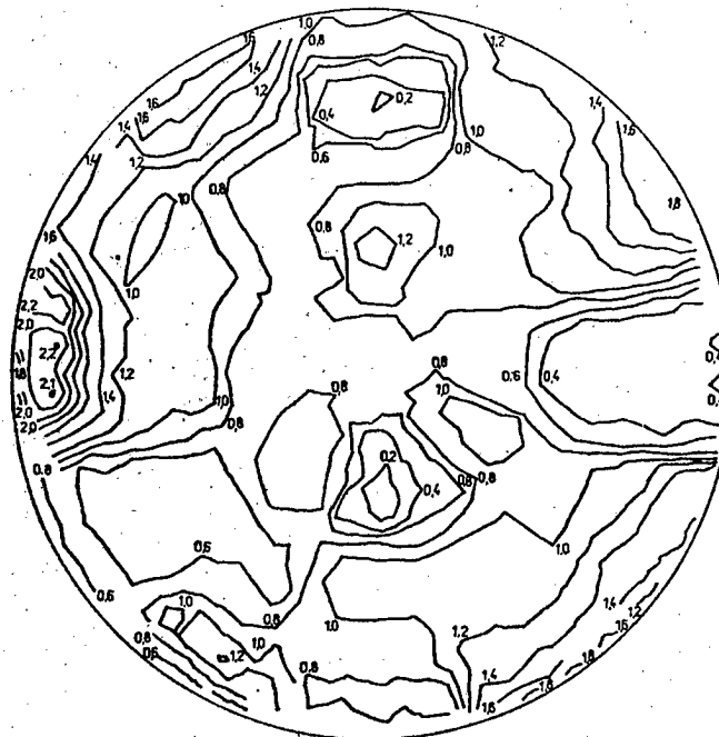
Figure 3. Results of Measurements on the Flow Distribution in a Model Generator
