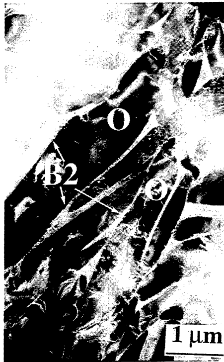
Figure 4.27 A bright field TEM image of the as-processed Ti-25Al-27Nb microstructure containing O and B2 laths; the longitudinal rod direction is horizontal.
