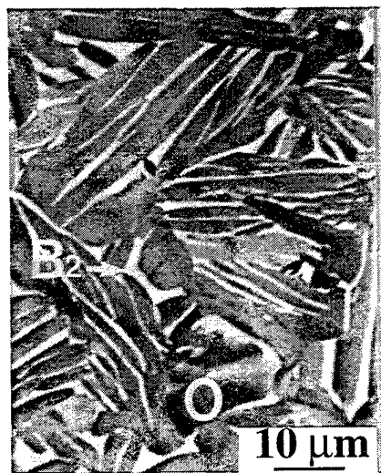
Figure 4.9 Ti-25Al-24Nb heat-treated sheet microstructures: (a) 875^\circ C/100h/WQ/900^\circ C/8h/WQ and (b) 975^\circ C/100h/WQ . These microstructures depict the effect of heat treatment on morphology.
