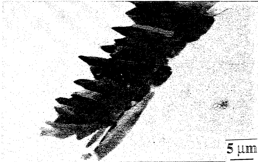
Figure 4.22 A high-magnification BSD SEM image of the aligned grain-boundary precipitates for a heat-treated (1090°C/0.5h/WQ/650°C/9h/WQ) Ti-23Al-27Nb sample.
