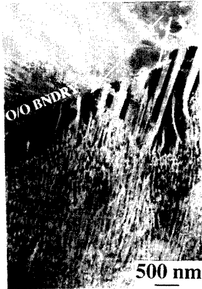
Figure 4.25 Microstructure of a 1090°C solutionized Ti-23Al-27Nb sample which was aged at 650°C for 681 hours depicting discontinuous precipitation resulting in coarser platelets at O/O boundaries.
