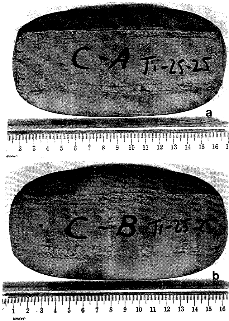
Figure 3.11 The can assemblies of the two uniformly deformed Ti-25Al-25Nb pancakes after the second forging runs.
