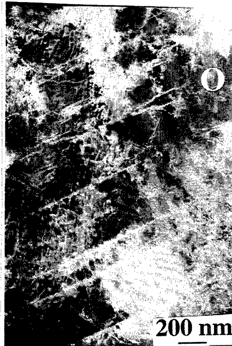
Figure 4.61 The deformed Ti-25Al-27Nb as-processed microstructure tested at 394 MPa/760°C. Dislocations formed within O grains in slip bands.
