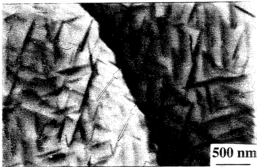
Figure 4.75 The deformation behavior for a heat treated (900°C/5h/WQ/650°C/55h/WQ) Ti-12Al-38Nb microstructure which was strained to more than 12% at RT. Wavy \beta slip traces readily transgressed O-phase platelets, indicated by the arrows.
