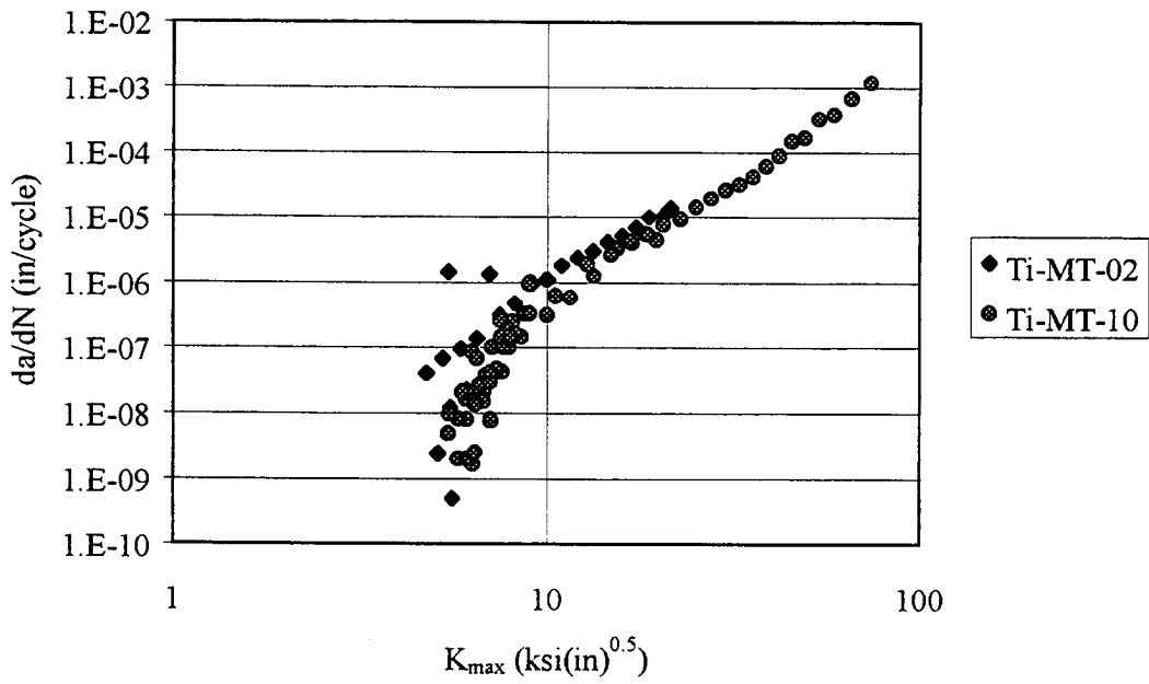
Figure 7: Crack Growth Rate Plot of Ti-6-4 Center Cracked Panels Using the Decreasing K Method with R=0.1 .
