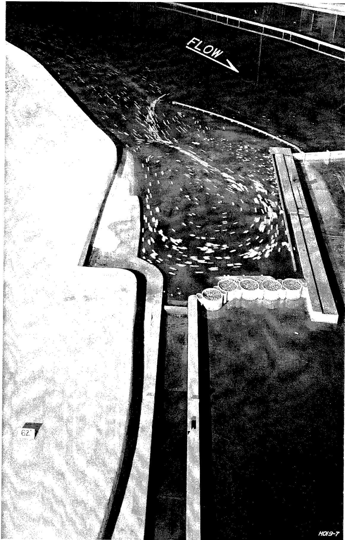
Photo 2. Base Test, total riverflow = 62,000 cfs, powerhouse discharge = 62,000 cfs. Looking upstream, confetti showing surface current patterns
