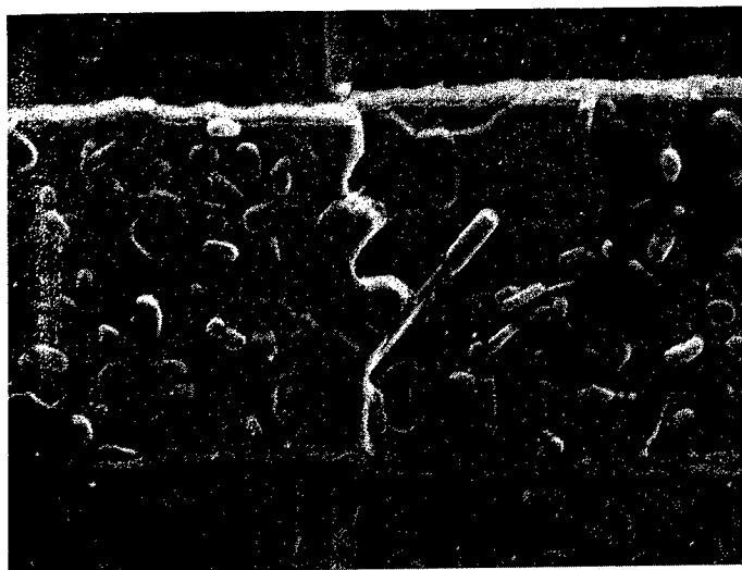
Fig. 4. SEM top view of a TBCCO step stack junction on a \text{LaAlO}_3 substrate ( bridge width 6\mu\text{m} )
