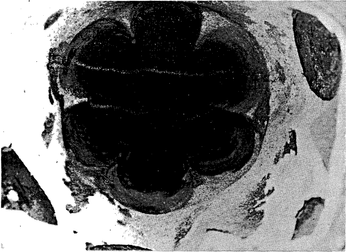
Figure 46. Photograph Showing Sharply Peaked Fuel Grain Spokes Following Run #35
