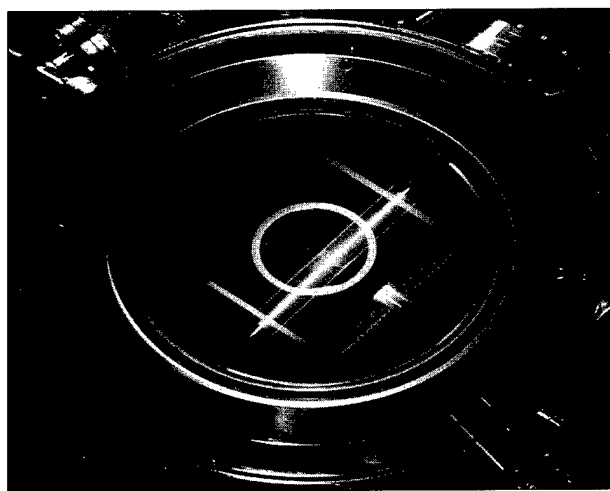
Above Isolated silicon epitaxy equipment. This equipment is used to produce silicon-on-insulator wafers for active matrix liquid crystal displays, high-temperature microsensors, and radiation-hardened static random access memory circuits.
