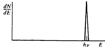
Figure 2.6 The differential distribution of electron kinetic energy for a series of photoelectric absorption events. (Knoll, 1979)
