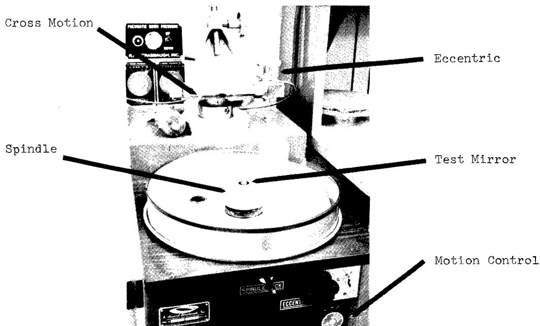
Fig. 7. Polishing Machine Showing Principal Components With Test Mirror Under Fabrication†
