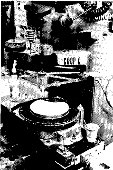
Fig. 21. Spindle and stroke mechanism of a CCOS machine.
