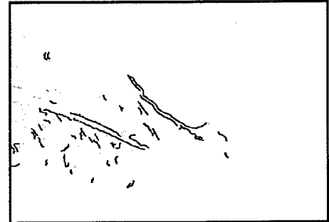
Fig 4b. Output of crack detection algorithm; cracks in black; non-cracks in gray.
