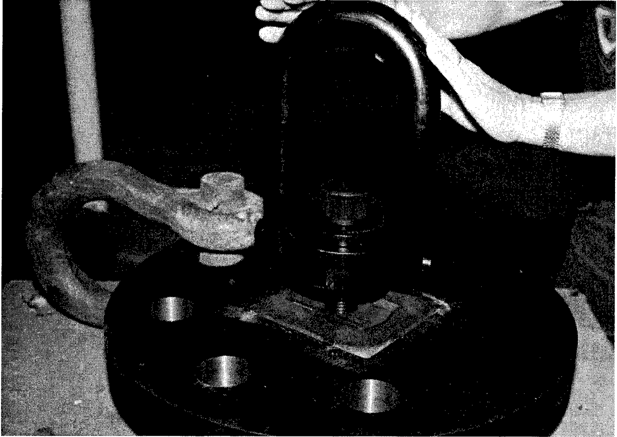
Figure 7. SHR Being Installed in ISO Anchor (NFESC # 9700127)
