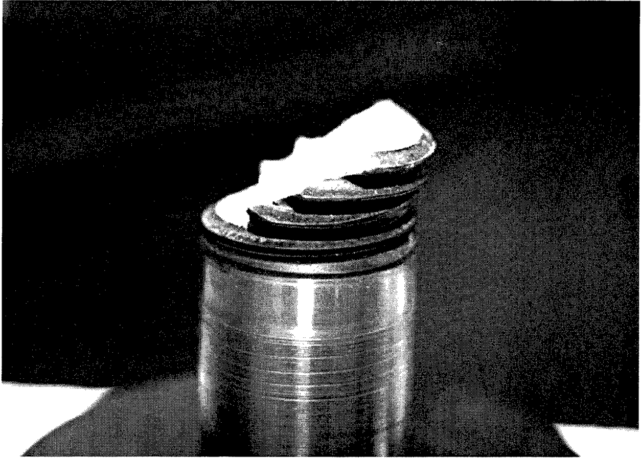
Figure 15. Bolt Failure at 119,000 Pounds (NFESC # 9700172)
