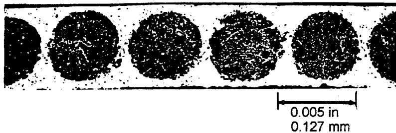
FIGURE 1.4. IDEALIZED LAMINA CROSS SECTION PERPENDICULAR TO THE FIBERS. This shows discrete yarns which are made up of a multiplicity of filaments.
