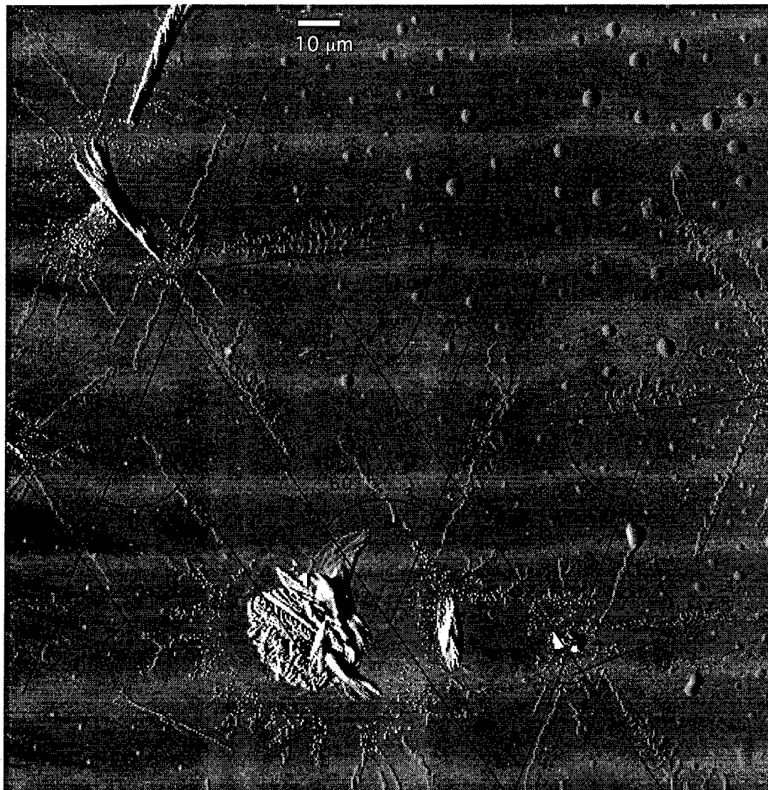
FIGURE 4.2. AFM image of the 2-D growth of GMS on mica at a large scale. The elongated crystal growth with six-fold symmetry indicates directional influence from the substrate.
