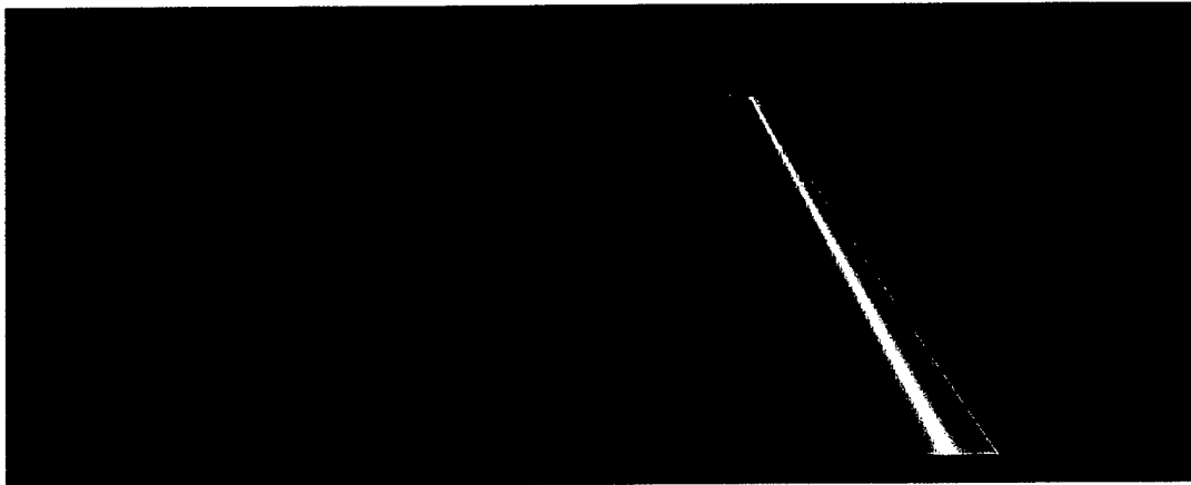
Fig. 7. Scattered E field (component parallel to ridge line) within the shadow pit at 131 MHz for H-polarized incident wave
