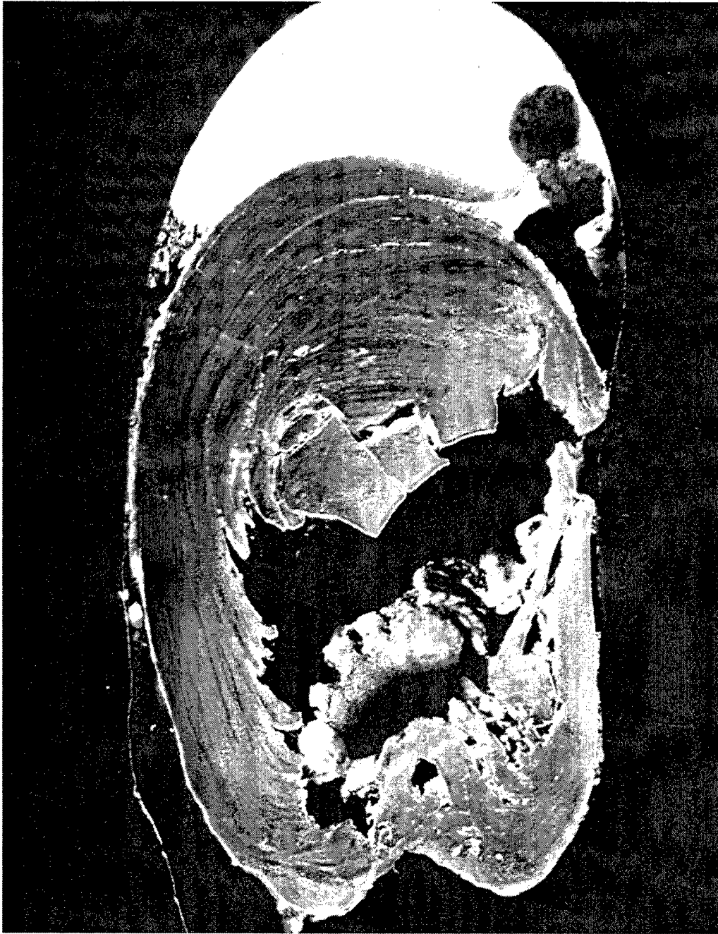
(a) Overview of Residual Penetrator (10 \times ).
