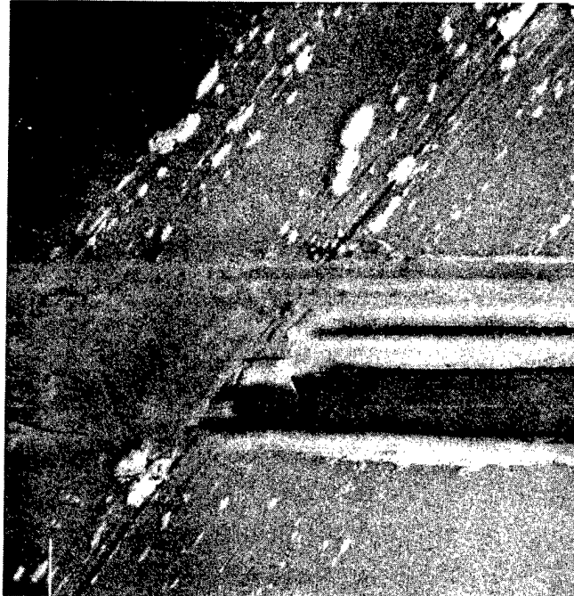
Fig. 21. Effect of surface flaw on scratching of zirconium/sapphire system. Scratch direction is from left to right. Scanning electron metallograph. 1600X.
