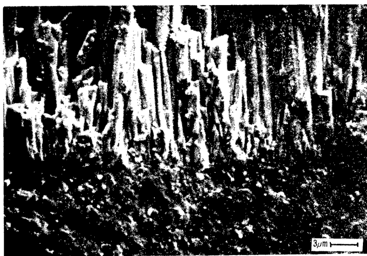
Figure 5. As-coated zirconia remained adherent to RBSN substrates with various pretreatments through flexure testing.
