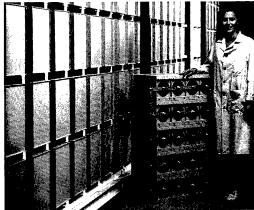
SDI research has led to dramatic reductions in size of high power capacitors
