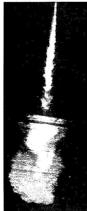
Figure 2: Evaporating spray illuminated with a dual intensity light sheet.
