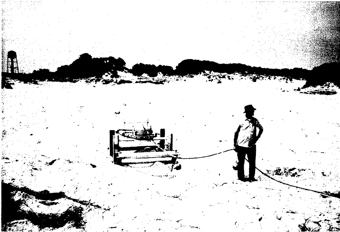
Figure 2. SUBSCAN system with tow sled being deployed from the beach. The towing frame, winch, and deployment system are designed for small research vessels and operation in high energy environments. The tow frame has been designed to be stable on the bottom while being towed slowly across the surf zone out to greater water depths. Outside the surf zone the vehicle will be flown in a traditional configuration while maintaining a constant depth above the seafloor..
