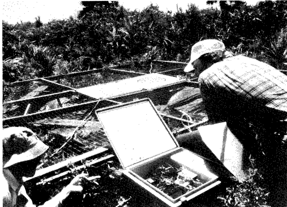
Figure 9. Dr. Paul Krehbiel (left) of New Mexico Tech. and Dr. Ewen Thomson (right) of the University of Florida inspect one of Dr. Thomson's VHF lightning detectors. Using an array of five such detectors, Dr. Thomson discovered the existence of pre- lightning sparks emanating from charged clouds.
