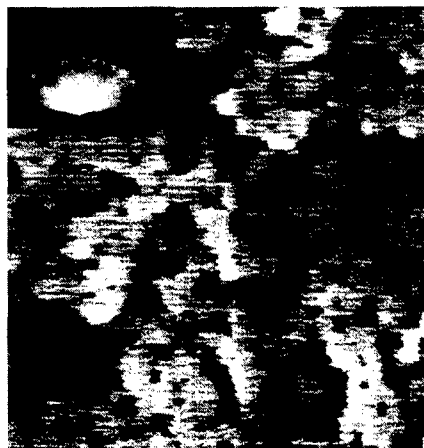
FIG. 4. 1 \times 1 \mu\text{m}^2 STM image of a Si sample initially containing a native oxide after an anneal at 800^\circ\text{C} for 10 min with a Si flux of 6 \text{ \AA/min} . A highly nonuniform surface results with a high density of large holes. The inset shows the corresponding RHEED pattern taken from this surface.
