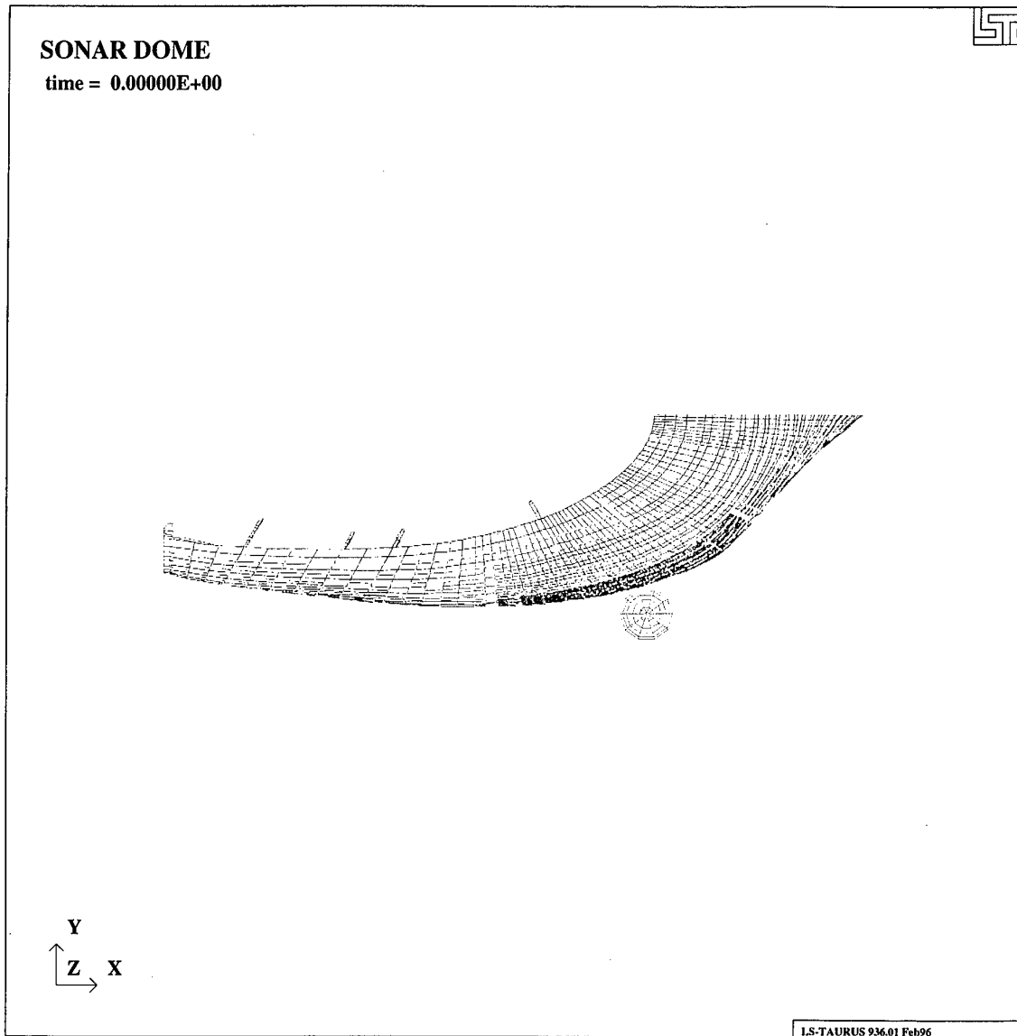
Figure 10 Mesh of the dome seen from the bottom in xy-plane (impacting sphere in blue)
