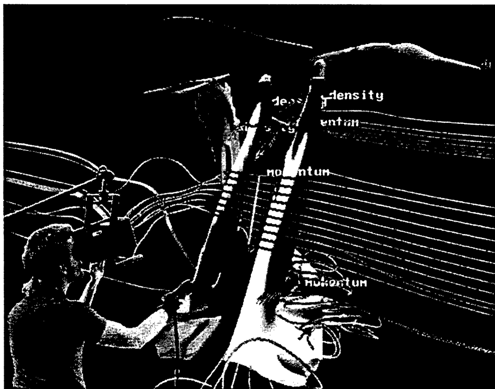
Figure 9: BOOM Use With NASA's Virtual Wind Tunnel
