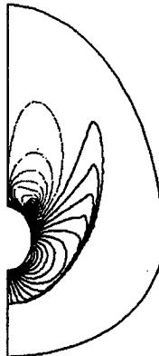
Fig.8. Isolines of velocity component along z in the flow around a cone at incidence.
