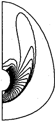
Fig.7. Pressure isolines for a flow around a cone at incidence.
