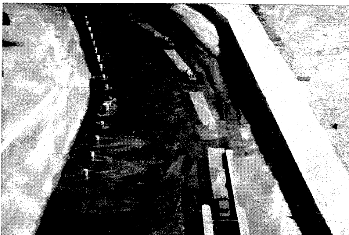
Photo 62. First stage of the dam cofferdam, 175-ft-wide navigation pass modified, looking downstream; discharge of 51,800 cfs; showing path of downbound tow leaving lock
