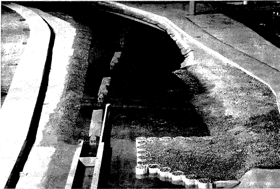
Photo 57. First stage of the dam cofferdam, 175-ft-wide navigation pass modified, looking upstream; discharge of 25,000 cfs; showing path of upbound tow leaving lock
