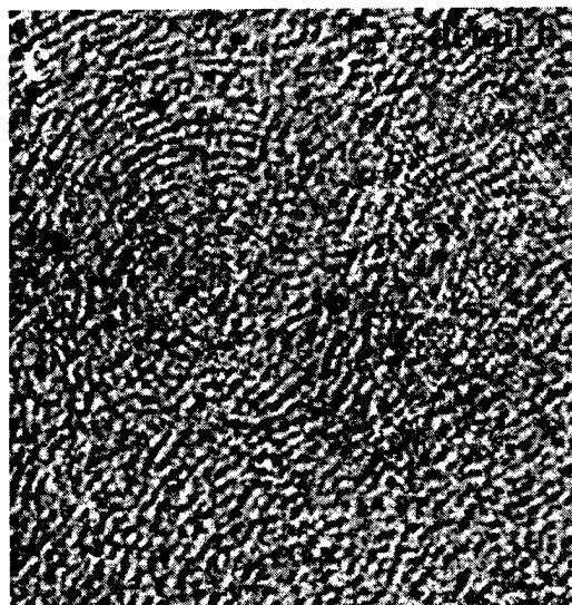
Figure 3: Note the arking in the FFT and the turbostratic appearance with circular symmetries of the PVD-carbon layer in the vicinity of the the SCS-6-fiber.
