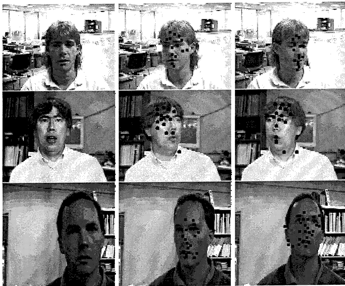
Figure 17: Examples of point matches. First column: model image. Other columns: matches between respective model image and other views of the object. Dots are LoG peaks that have been matched to model image peaks.
