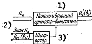
Figure 5. Structural Diagram of Element of Digital Fourier Transform Filter
