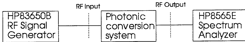
Figure 8. Measurement Setup for Conversion Gain.
