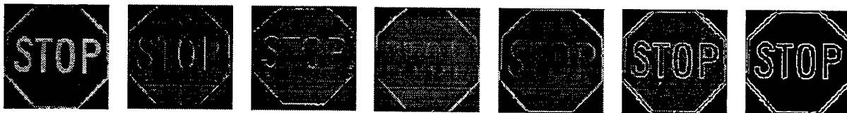
Figure 7: A stop sign, its partial derivatives with respect to x , y , \theta , and s = s_x = s_y , and its edge map and thresholded edge map.
