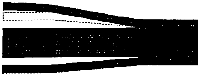
(a) brass cap (0,1) mode at 23.1 kHz
