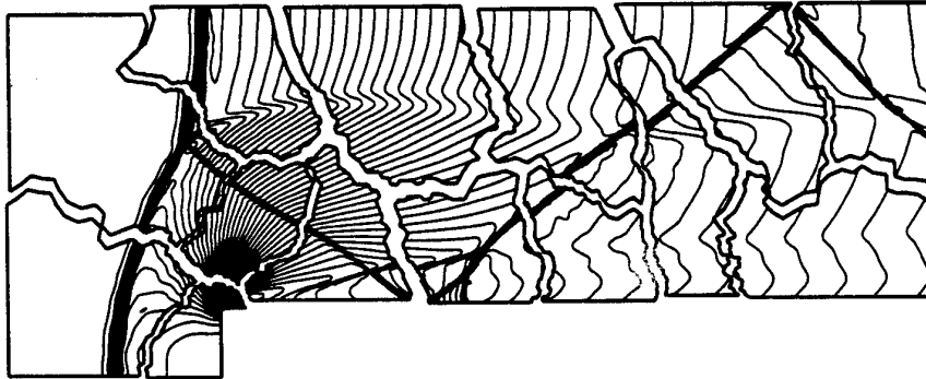
Fig. 7. Iso-density contours for Mach 3 inviscid Euler flow over a backward-facing step with exploded view of 16 subdomain partitioning.
