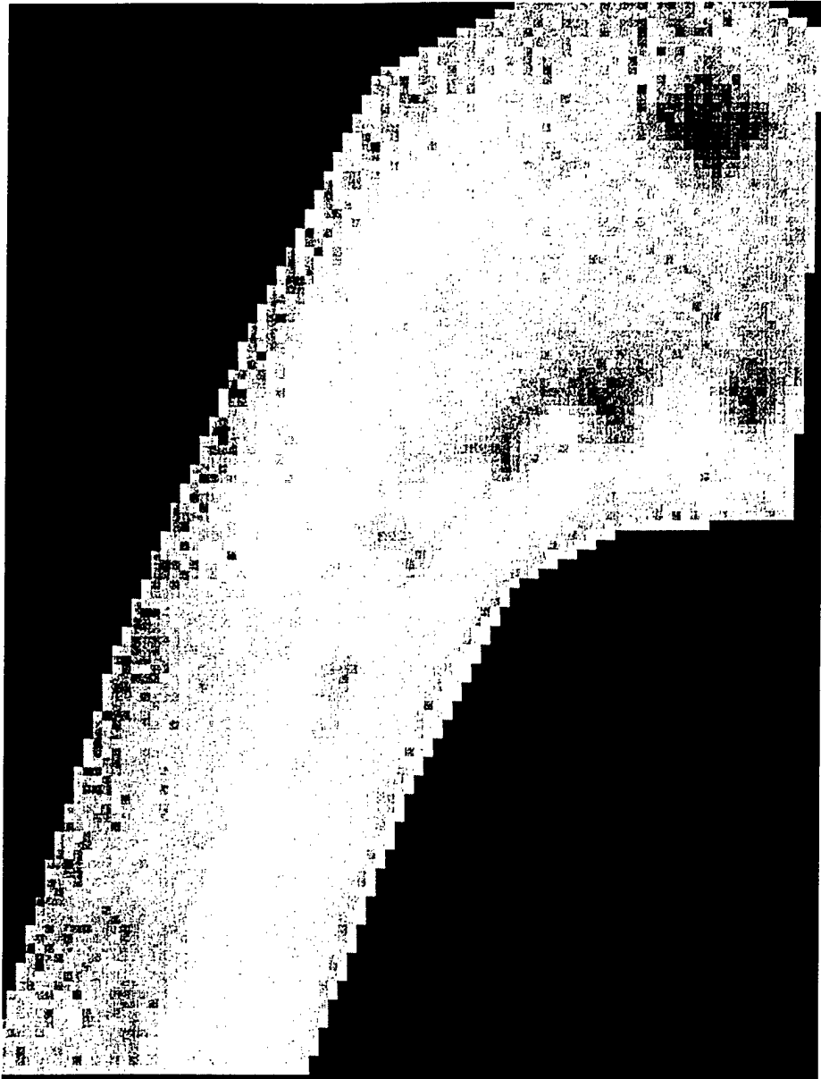
Figure 5.1.11-3. 3 MHz water jet through transmission ultrasonic image of "chainguard"
