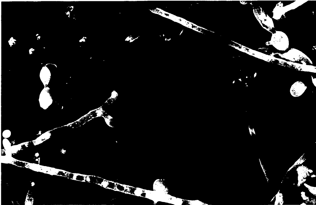
Figure 2. Scanning electron micrograph showing colonization and penetration of a fluorinated polyimide resin/carbon fiber composite by hyphae of fungi ( \times 2000 )
