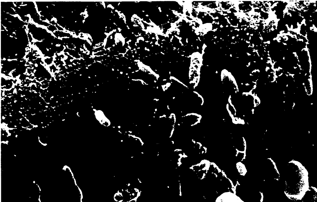
Figure 3. Scanning electron micrograph of a natural population of bacteria growing on the surface of a carbon fiber utilizing sizing chemical as carbon and energy sources ( \times 1000 )
