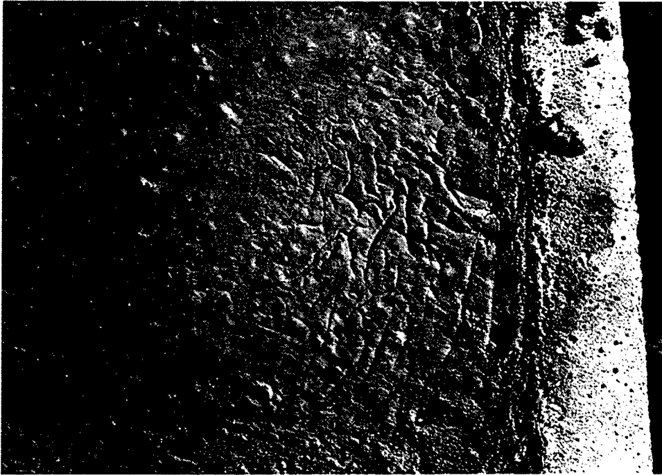
Figure 14. Very cohesive material (No. 10), sticky, difficult to finish (Florida)
