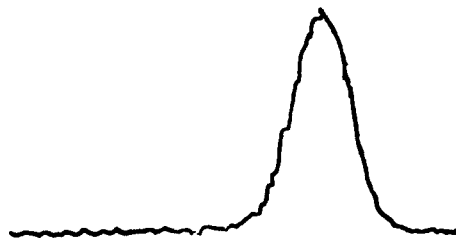
(b) light pulse from a single longitudinal mode laser
