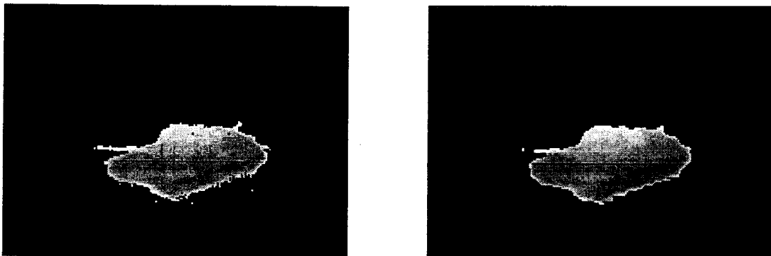
Figure 5.1 Height images produced by opel3d computer program. Left is with no median processing. Right is with double median processing
