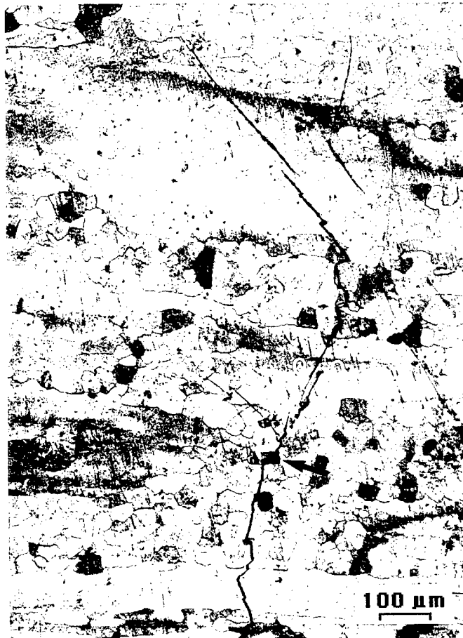
Fig. 1 Optical microscope view of the crack path through one of the two specimens. Loading axis was horizontal and crack growth was from bottom to top. Below the arrow, crack was grown by cyclic loading, R = 0.1 , and above the arrow, the crack was grown by monotonic loading. EBSD patterns were made in large grains at the locations shown.
